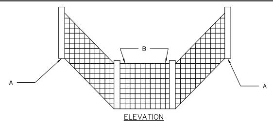
POINTS 'A' SHOULD BE HIGHER THAN POINTS 'B' IF SLOPE DICTATES
