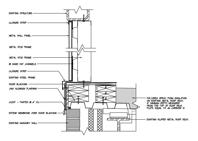
NOTE: INSTALL METAL WALL PENEL AT INSIDE FACE OF ENTRY GABLE. APPROX. 95-0' ON THREE SIDES OF ENTRY.
