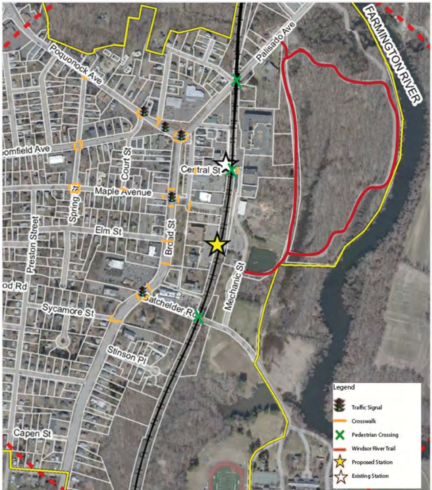
Figure 13. Pedestrian and Bicycle Facilities
