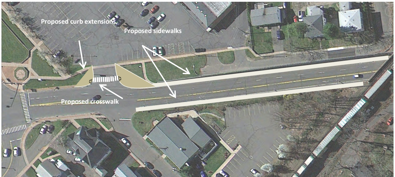
Figure 18. Pedestrian Facilities on Palisado Avenue
